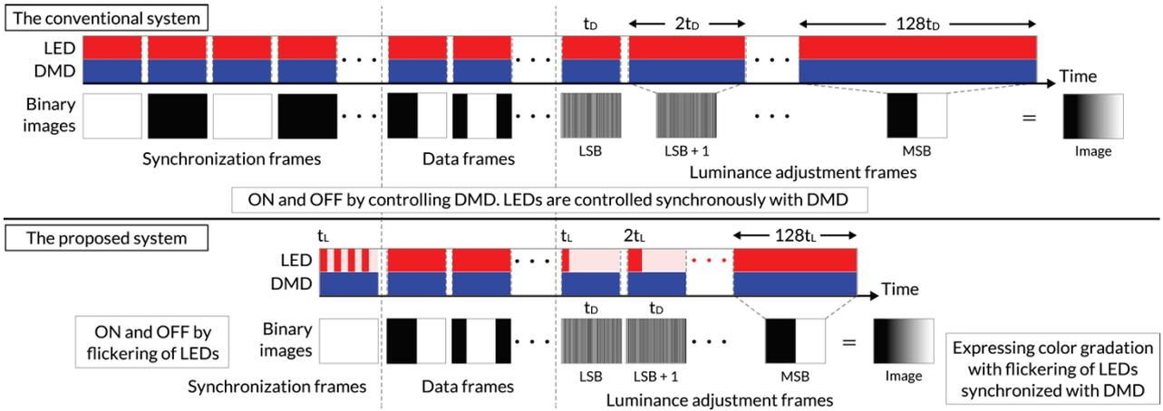
**Fig. 5 Comparison of the data structure, DMD, and LED light sources control between the conventional and proposed system.  $t_D$  is the minimum update time of the DMD and  $t_L$  is the unit flickering time of the LED light sources.**
