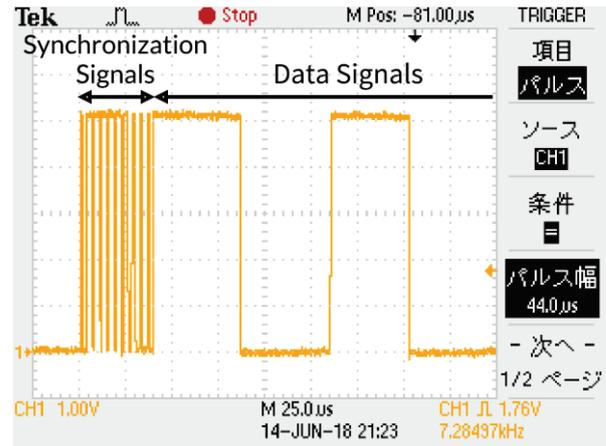
Fig. 8 The synchronization and data signal
