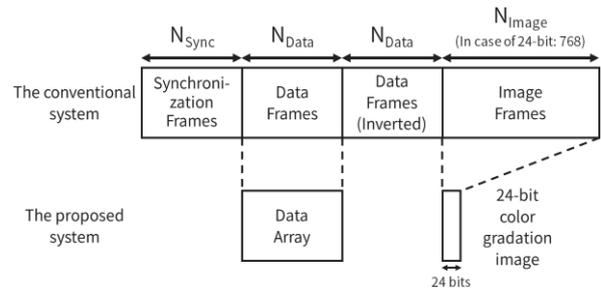
**Fig. 4 Amount of transferred data in the conventional system and proposed system.  $N_{Sync}$ ,  $N_{Data}$ ,  $N_{Image}$  are the number of bits of the synchronization signal, transmission data, and color gradation, respectively.**
